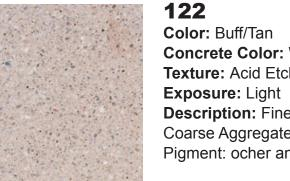
Concrete Color: White Texture: Acid Etched **Description:** Fine Aggregate: crushed White limestone; Coarse Aggregate: 3/8 to 1/8 in. White limestone; Pigment: ocher and black
