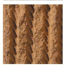
**577** Color: Yellow Concrete Color: White Finish: Standard Fractured Rope Description: Fine Aggregate: reddish brown concrete sand; Coarse Aggregate: 3/8 to 1/8 in. reddish brown river gravel; Pigment: yellow
