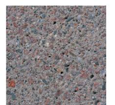
**366** Color: Pink Concrete Color: Gray Texture: Sandblasted Exposure: Medium Description: Fine Aggregate: crushed buff limestone; Coarse Aggregate: 70% - 9/16 to 3/16 in. red granite, 30% - 3/8 to 1/8 in. black granite
