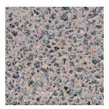
Color: Black - Buff/Tan Concrete Color: White Texture: Sandblasted Exposure: Medium Description: Fine Aggregate: off-White river sand, Coarse Aggregate: 1/2 to 1/4 in. black granite, Pigment: dark buff
