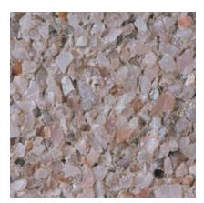
Color: Pink Concrete Color: White Texture: Retarded Exposure: Medium Description: Fine Aggregate: crushed rose quartz; Coarse Aggregate: 5/8 to 9/32 in. rose quartz
