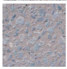
**103** Color: Grey Concrete Color: White Texture: Sandblasted Exposure: Medium Description: Fine Aggregate: White masonry sand; Coarse Aggregate: light green marble; Pigment: green
