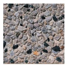
Color: Grey Concrete Color: White Texture: Retarded Exposure: Medium Description: Fine Aggregate: crushed gray quartz; Coarse Aggregate: 90% - 1/2 to 1/4 in. gray quartz, 10% - 3/8 to 1/8 in. black granite
