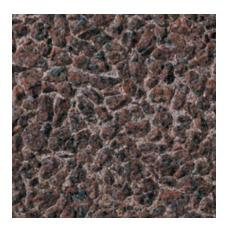
Color: Red Concrete Color: White Texture: Retarded Exposure: Medium Description: Fine Aggregate: 50% - reddish brown masonry sand, 50% - crushed red granite; Coarse Aggregate: 9/16 to 3/16 in. red granite; Pigment: red
