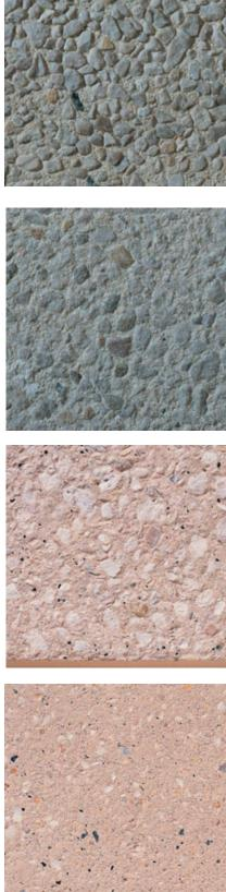
Color: White Concrete Color: White Texture: Retarded Exposure: Medium **Description:** Fine Aggregate: crushed White quartz; Coarse Aggregate: 1/2 to 1/4 in. White quartzite
