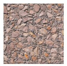
Color: Buff/Tan Concrete Color: antique White Texture: Sandblasted Exposure: Medium Description: Fine Aggregate: crushed buff limestone, Coarse: 1/2 to 1/4 in. buff limestone
