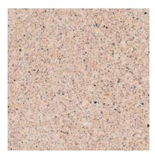
Color: Buff/Tan Concrete Color: White Texture: Acid Etched Exposure: Medium Description: Fine Aggregate: buff masonry sand; Coarse Aggregate: 3/8 to 1/8 in. buff limestone
