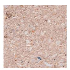
197 Color: Buff/Tan Concrete Color: White Texture: Sandblasted Exposure: Deep **Description:** Fine Aggregate: crushed White limestone; Coarse Aggregate: 1/2 to 1/4 in. buff limestone; Pigment: buff
