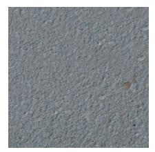
Color: Grey Concrete Color: White Texture: Sandblasted Exposure: Light Description: Fine Aggregate: crushed gray limestone; Coarse Aggregate: 1/2 in. gray limestone, Pigment: brown
