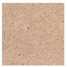
272 Color: Buff/Tan Concrete Color: White Texture: Acid Etched Exposure: Light Description: Fine Aggregate: buff masonry sand; Coarse Aggregate: 3/8 to 1/8 in. buff limestone; Pigment: buff
