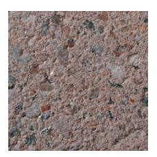
Color: Pink Concrete Color: White Texture: Sandblasted Exposure: Medium Description: Fine Aggregate: crushed pink feldspar; Coarse Aggregate: 5/8 to 9/32 in. pink feldspar; Pigment: red
