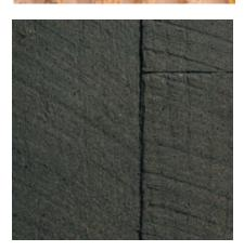
**581** Color: Grey Concrete Color: Gray Finish: Extra Rough Sawn Description: Fine Aggregate: reddish brown concrete sand; Coarse Aggregate: 3/8 to 1/8 in. reddish brown river gravel; Pigment: red
