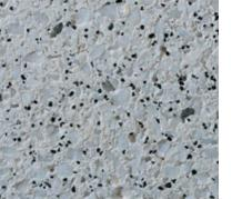
145 Color: White Concrete Color: White Texture: Sandblasted **Exposure:** Light **Description:** Fine Aggregate: crushed White quartz; Coarse Aggregate: 80% - 3/8 to 1/8 White guartz, 10% - 3/8 to 1/8 in. black granite, 10% - black slag
