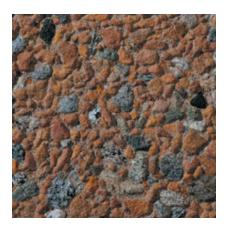
Color: Brown Concrete Color: Gray Texture: Sandblasted Exposure: Medium Description: Fine Aggregate: reddish brown masonry sand; Coarse Aggregate: 50% - 1/2 to 1/4 in. gray granite, 50% - 1/2 to 1/4 in. buff river gravel; Pigment: brown
