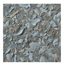
Color: White Concrete Color: 93% - White; 7% - Gray Texture: Retarded Exposure: Deep Description: Fine Aggregate: White masonry sand; Coarse Aggregate: crushed oyster shell
