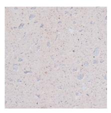
**117** Color: White Concrete Color: White Texture: Sandblasted Exposure: Light Description: Fine Aggregate: White concrete sand; Coarse Aggregate: 1/2 to 1/4 in. gray limestone; Pigment: dark buff and dark gray
