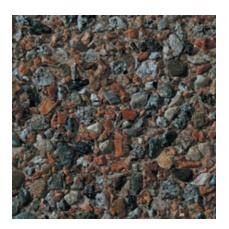
Color: Brown Concrete Color: 60% - White; 40% - Gray Texture: Retarded Exposure: Medium Description: Fine Aggregate: crushed pink feldspar, Coarse Aggregate: 70% - 1/2 to 1/4 in. gray granite, 30% - 5/8 to 9/32 in. pink feldspar
