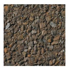
Color: Brown Concrete Color: Gray Texture: Retarded Exposure: Light Description: Fine Aggregate: crushed tan limestone; Coarse Aggregate: 5/8 to 1/4 in. tan limestone; Pigment: yellow
