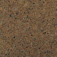
Color: Brown Concrete Color: White Texture: Acid Etched Exposure: Medium Description: Fine Aggregate: reddish brown concrete sand, Coarse Aggregate: 1/2 in. reddish brown river gravel, Pigment: yellow
