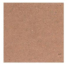
Color: Brown Concrete Color: White Texture: Acid Etched Exposure: Light Description: Fine Aggregate: buff crushed limestone; Coarse Aggregate: 1/2 to 1/4 in. buff limestone; Pigment: ocher
