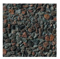
**465** Color: Red Concrete Color: White Texture: Retarded Exposure: Medium Description: Fine Aggregate: crushed gray granite; Coarse Aggregate: 75% - 5/8 to 9/32 in. red granite, 25% - 5/8 to 9/32 in. gray granite; Pigment: black
