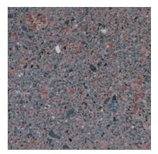
Color: Pink - Grey Concrete Color: Gray Texture: Sandblasted Exposure: Light Description: Fine Aggregate: 70% - crushed black granite, 30% - black granite grit; Coarse Aggregate: 70% - 1/2 to 1/4 in. red granite, 30% - 1/2 to 1/4 in. black granite; Pigment: red
