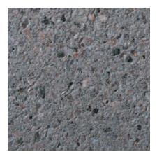
Color: Pink Concrete Color: Gray Texture: Sandblasted Exposure: Light Description: Fine Aggregate: crushed red quartzite; Coarse Aggregate: 60% - 3/8 to 1/8 in. pink feldspar, 30% - 3/8 to 1/8 in. black granite, 10% - 3/8 to 1/8 in. red quartzite
