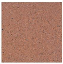
**368** Color: Brown Concrete Color: 70% - Gray; 30% - White Texture: Acid Etched Exposure: Light Description: Fine Aggregate: crushed brown granite; Coarse Aggregate: 1/2 to 1/4 in. black granite; Pigment: buff and orange
