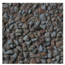
293A Color: Brown Concrete Color: Gray Texture: Sandblasted Exposure: Deep Description: Fine Aggregate: crushed brown limestone; Coarse Aggregate: 3/8 to 1/8 in. brown limestone; Pigment: brown
