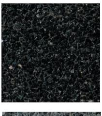
Color: Black Concrete Color: Gray Texture: Retarded Exposure: Light Description: Fine Aggregate: crushed black granite; Coarse Aggregate: 9/32 to 1/8 in. black granite
