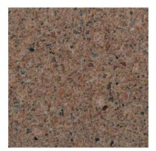
Color: Red Concrete Color: White Texture: Acid Etched Exposure: Medium Description: Fine Aggregate: reddish brown concrete sand; Coarse Aggregate: 3/8 to 1/8 in. reddish brown river gravel; Pigment: yellow
