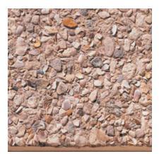
Color: Buff/Tan Concrete Color: White Texture: Retarded Exposure: Medium **Description:** Fine Aggregate: crushed White limestone; Coarse Aggregate: 1/2 to 1/4 in. buff limestone; Pigment: buff
