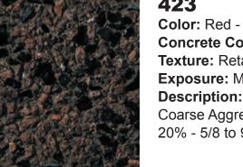
Color: Red - Black Concrete Color: Gray Texture: Retarded Exposure: Medium **Description:** Fine Aggregate: crushed red granite; Coarse Aggregate: 80% - 5/8 to 9/32 in. red granite, 20% - 5/8 to 9/32 in. black granite
