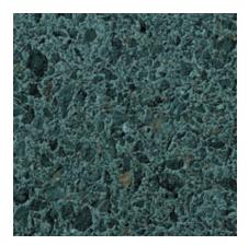
Color: Green Concrete Color: White Texture: Acid Etched Exposure: Light Description: Fine Aggregate: crushed green marble; Coarse Aggregate: 1/2 to 1/4 in. green marble; Pigment: green
