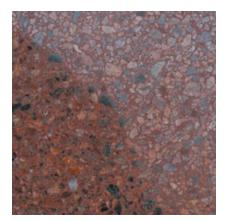
Color: Red Concrete Color: Gray Finish: Polished Description: Finish Aggregate: crushed red granite; Coarse Aggregate: 5/8 to 1/8 in. red granite; Pigment: tannish pink
