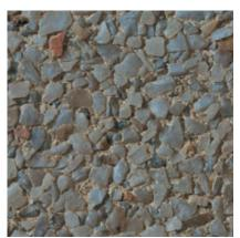
233 Color: White Concrete Color: White Texture: Retarded Exposure: Medium Description: Fine Aggregate: crushed White quarts; Coarse Aggregate: 5/8 to 9/32 in. White quartz; Pigment: yellow
