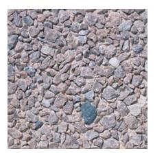
**116** Color: Buff/Tan Concrete Color: White Texture: Retarded Exposure: Medium Description: Fine Aggregate: White concrete sand; Coarse Aggregate: 1/2 to 1/4 in. gray limestone; Pigment: dark buff and dark gray
