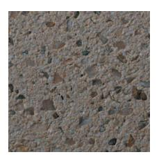
Color: White Concrete Color: White Texture: Sandblasted Exposure: Medium Description: Fine Aggregate: crushed White marble; Coarse Aggregate: 60% - 1/2 to 1/4 in. amber quartz, 40% - 1/2 to 1/4 in. White quartz
