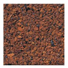
Color: Red Concrete Color: 50% - White; 50% - Gray Texture: Retarded Exposure: Medium Description: Fine Aggregate: crushed black granite; Coarse Aggregate: 1/2 to 1/4 in. reddish brown limestone; Pigment: orange
