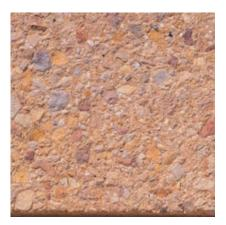
**320** Color: Buff/Tan Concrete Color: White Texture: Sandblasted Exposure: Medium Description: Fine Aggregate: buff concrete sand; Coarse Aggregate: 3/4 to 1/8 in. buff limestone ; Pigment: buff
