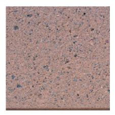
Color: Brown Concrete Color: 70% - White; 30% - Gray Texture: Sandblasted Exposure: Medium Description: Fine Aggregate: crushed brown granite; Coarse Aggregate: 1/2 to 1/4 in. pink granite; Pigment: reddish brown and yellow
