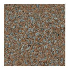
Color: Brown Concrete Color: White Texture: Acid Etched Exposure: Deep Description: Fine Aggregate: reddish brown concrete sand; Coarse Aggregate: 3/8 to 1/8 in. gray granite; Pigment: buff
