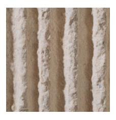
Color: White Concrete Color: White Finish: Simulated Bushhammer Description: Fine Aggregate: crushed White marble; Coarse Aggregate: 5/8 to 9/32 in. White marble
