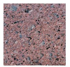
**363B** Color: Pink Concrete Color: White Texture: Sandblasted Exposure: Light Description: Fine Aggregate: crushed red granite; Coarse Aggregate: 1/2 to 1/4 in. pink granite; Pigment: red
