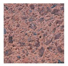
**364B** Color: Pink Concrete Color: White Texture: Sandblasted Exposure: Light Description: Fine Aggregate: crushed red granite; Coarse Aggregate: 1/2 to 1/8 in. red granite; Pigment: red
