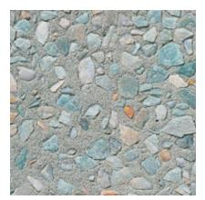
Color: Green Concrete Color: White Texture: Sandblasted Exposure: Medium Description: Fine Aggregate: silica sand; Coarse Aggregate: 1/2 to 1/4 in. green quartzite; Pigment: green
