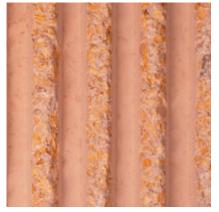
**579** Color: Yellow Concrete Color: White Finish: Bushhammered Rib Description: Fine Aggregate: crushed yellow marble; Coarse Aggregate: 5/8 to 9/32 in. yellow marble
