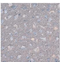
**181** Color: Grey Concrete Color: 50% - White; 50% - Gray Texture: Sandblasted Exposure: Light Description: Fine Aggregate: White silica sand; Coarse Aggregate: 1/2 to 1/4 in. blue gray limestone; Pigment: dark gray
