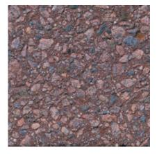
Color: Red Concrete Color: Gray Texture: Sandblasted Exposure: Medium Description: Fine Aggregate: crushed brown granite; Coarse Aggregate: 1/2 to 1/4 in. pink granite; Pigment: reddish orange and red
