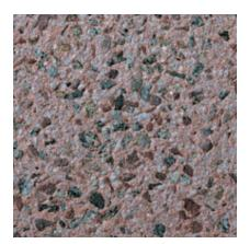
Color: Pink Concrete Color: White Texture: Sandblasted Exposure: Light Description: Fine Aggregate: crushed White marble; Coarse Aggregate: 80% - 1/2 to 1/4 in. gray granite, 20% - 9/32 to 1/8 in red quartzite; Pigment: red
