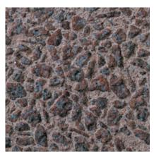
**394** Color: Pink Concrete Color: White Texture: Sandblasted Exposure: Medium Description: Fine Aggregate: 50% - reddish brown masonry sand, 50% - crushed red granite; Coarse Aggregate: 9/16 to 3/16 in. red granite; Pigment: red
