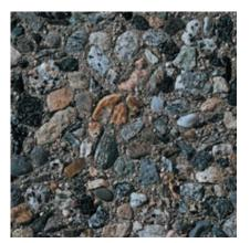
**477** Color: Grey Concrete Color: Gray Texture: Retarded Exposure: Medium Description: Fine Aggregate: crushed gray granite; Coarse Aggregate: 1/2 to 1/4 in. gray granite
