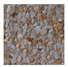
Color: White Concrete Color: White Texture: Retarded Exposure: Medium Description: Fine Aggregate: crushed White quartz, Coarse Aggregate: 80% - 5/8 to 9/32 in. White quartz, 20% - 1/2 to 1/4 in. amber quartz; Pigment: yellow
