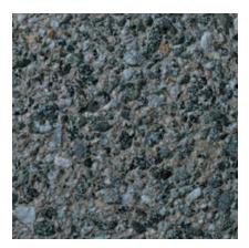
Color: Grey Concrete Color: Gray Texture: Sandblasted Exposure: Medium Description: Fine Aggregate: crushed gray granite; Coarse Aggregate: 1/2 to 1/4 in. gray granite
