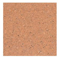
Color: Buff/Tan Concrete Color: White Texture: Sandblasted Exposure: Medium Description: Fine Aggregate: reddish brown concrete sand; Coarse Aggregate: 1/2 to 1/4 in. multicolored river gravel; Pigment: yellow
