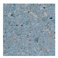
Color: Blue Concrete Color: White Texture: Sandblasted Exposure: Medium Description: Fine Aggregate: crushed green quartzite; Coarse Aggregate: 9/16 to 3/16 in. green quartzite; Pigment: blue
