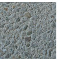
129 Color: White Concrete Color: White **Texture:** Sandblasted Exposure: Medium Description: Fine Aggregate: crushed White quartz; Coarse Aggregate: 1/2 to 1/4 in. White quartzite
