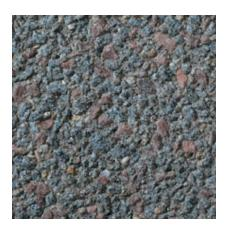
Color: Pink - Grey Concrete Color: Gray Texture: Sandblasted Exposure: Medium Description: Fine Aggregate: crushed gray granite; Coarse Aggregate: 80% - 3/8 to 1/8 in. gray granite, 20% - 3/8 to 1/8 in. pink quartzite; Pigment: red
