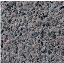
**390** Color: Pink Concrete Color: White Texture: Sandblasted Exposure: Light Description: Fine Aggregate: crushed pink granite; Coarse Aggregate: 1/2 to 1/8 in. pink granite ; Pigment: red
