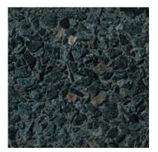
**533** Color: Black Concrete Color: Gray Texture: Retarded Exposure: Medium Description: Fine Aggregate: crushed black granite; Coarse Aggregate: 1/2 to 1/4 in. black granite
