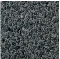
**547** Color: Grey Concrete Color: Gray Texture: Sandblasted Exposure: Light Description: Fine Aggregate: crushed black granite; Coarse Aggregate: 9/32 to 1/8 in. black granite
