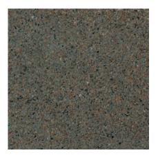
Color: Brown Concrete Color: Gray Texture: Acid Etched Exposure: Light Description: Fine Aggregate: reddish brown concrete sand; Coarse Aggregate: 3/8 to 1/8 in. reddish brown river gravel
