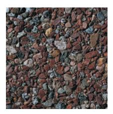
Color: Red Concrete Color: Gray Texture: Retarded Exposure: Medium Description: Fine Aggregate: crushed gray granite; Coarse Aggregate: 60% - 1/2 to 1/4 in. gray granite, 40% - 9/32 to 1/8 in. red quartzite; Pigment: red
