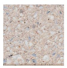
Color: Buff/Tan Concrete Color: White Texture: Sandblasted Exposure: Medium Description: Fine Aggregate: buff concrete sand; Coarse Aggregate: 1/2 to 1/4 in. brown limestone; Pigment: buff
