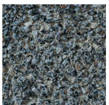
**509** Color: Grey Concrete Color: White Texture: Retarded Exposure: Medium Description: Fine Aggregate: crushed gray granite; Coarse Aggregate: 3/8 to 1/8 in. gray granite; Pigment: yellow
