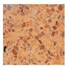
**561** Color: Buff/Tan Concrete Color: White Finish: Polished Description: Fine Aggregate: buff masonry sand; Coarse Aggregate: 50% - 3/4 to 3/8 in. buff limestone, 50% - 3/4 to 3/8 in. brownish red limestone; Pigment: buff
