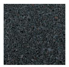
Color: Black Concrete Color: White **Texture:** Sandblasted **Exposure:** Medium **Description:** Fine Aggregate: crushed gray traprock; Coarse Aggregate: 1/2 to 1/4 in. gray traprock; Pigment: black
