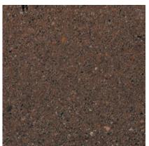
Color: Brown Concrete Color: Gray Texture: Acid Etched Exposure: Light Description: Fine Aggregate: reddish brown concrete sand; Coarse Aggregate: 3/8 to 1/8 in. reddish brown river gravel; Pigment: brown
