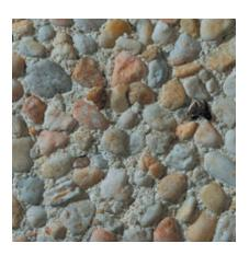
Color: White Concrete Color: White Texture: Retarded Exposure: Deep Description: Fine Aggregate: White river sand ; Coarse Aggregate: 7/8 to 9/16 in. White river gravel
