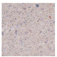
**169** Color: Pink Concrete Color: White Texture: Sandblasted Exposure: Medium Description: Fine Aggregate: crushed gray quartz, Coarse Aggregate: 1/2 to 1/4 in. pink marble
