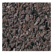
**521** Color: Brown Concrete Color: Gray Texture: Retarded Exposure: Medium Description: Fine Aggregate: 80% - crushed light purple quartzite, 20% - crushed black granite; Coarse Aggregate: 3/8 to 1/8 in. light purple quartzite; Pigment: black
