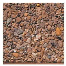
Color: Brown Concrete Color: White Texture: Retarded Exposure: Medium Description: Fine Aggregate: buff concrete sand; Coarse Aggregate: 1/2 to 1/4 in. buff limestone; Pigment: brown
