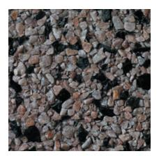
Color: Pink - Black Concrete Color: Gray Texture: Retarded Exposure: Medium Description: Fine Aggregate: crushed red quartzite; Coarse Aggregate: 75% - 1/8 to 1/8 in. flamingo quartz, 25% - 5/8 to 9/32 in. black granite; Pigment: red
