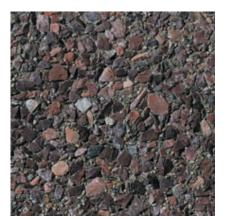
**453** Color: Red Concrete Color: Gray Texture: Retarded Exposure: Medium Description: Fine Aggregate: crushed gray granite; Coarse Aggregate: 3/8 to 1/8 in. red marble
