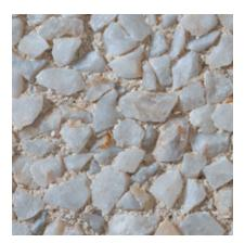
Color: White Concrete Color: White Texture: Retarded Exposure: Deep **Description:** Fine Aggregate: crushed White quartz; Coarse Aggregate: 7/8 to 5/8 in. White quartz
