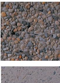
Color: White Concrete Color: White Texture: Retarded Exposure: Medium Description: Fine Aggregate: White masonry sand; Coarse Aggregate: 1/2 to 1/4 in. White river gravel
