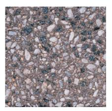
**336** Color: White - Brown Concrete Color: White Texture: Sandblasted Exposure: Medium Description: Fine Aggregate: White concrete sand; Coarse Aggregate: 50% - 3/8 to 1/8 in. White limestone 50% - 3/8 to 1/8 in. salt and pepper granite; Pigment: brown
