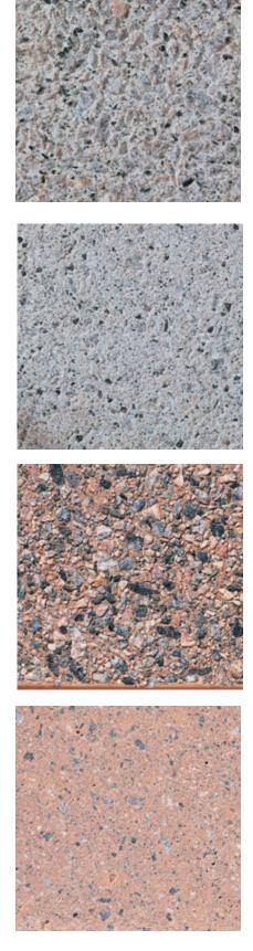
Color: Grey Concrete Color: White Texture: Retarded Exposure: Medium Description: Fine Aggregate: 75% - crushed gray granite, 25% - crushed black granite grit; Coarse Aggregate: 5/8 to 9/32 in. gray granite; Pigment: black
