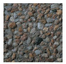
Color: Brown Concrete Color: Gray Texture: Sandblasted Exposure: Medium Description: Fine Aggregate: reddish brown concrete sand; Coarse Aggregate: 60% - 1/2 to 1/4 in. amber quartz, 40% - 3/8 to 1/8 in. reddish brown river gravel
