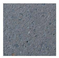
Color: Grey Concrete Color: Gray Texture: Sandblasted Exposure: Light Description: Fine Aggregate: crushed blue marble; Coarse Aggregate: 1/2 to 1/8 in. blue marble
