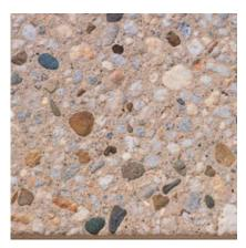
214 Color: Buff/Tan Concrete Color: Antique White Texture: Sandblasted Exposure: Deep Description: Fine Aggregate: reddish brown concrete sand; Coarse Aggregate: 80% - 3/4 to 3/8 in. buff, river gravel, 20% - 5/8 to 3/8 in. multicolor, river gravel
