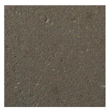
**268** Color: Brown Concrete Color: 70% - Gray; 30% - White Texture: Sandblasted Exposure: Light Description: Fine Aggregate: crushed reddish brown limestone; Coarse Aggregate: 5/8 to 9/32 in. reddish brown limestone; Pigment: buff
