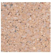
**187** Color: Buff/Tan Concrete Color: White Texture: Sandblasted Exposure: Medium Description: Fine Aggregate: buff concrete sand; Coarse Aggregate: 1/2 to 1/4 in. buff limestone; Pigment: brown
