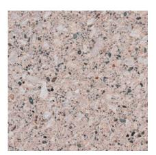
**149** Color: Buff/Tan Concrete Color: White Texture: Sandblasted Exposure: Medium Description: Fine Aggregate: crushed buff limestone, Coarse Aggregate: 1/2 to 1/4 in. White limestone
