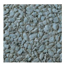
Color: White Concrete Color: White Texture: Retarded Exposure: Medium Description: Fine Aggregate: crushed gray granite; Coarse Aggregate: 5/8 to 9/32 in. White marble
