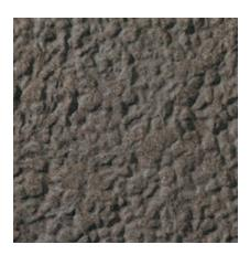
Color: Grey Concrete Color: Gray Finish: Simulated Bushhammer Description: Fine Aggregate: reddish brown concrete sand; Coarse Aggregate: 3/8 to 1/8 in. reddish brown river gravel
