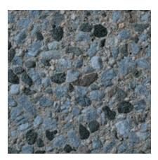
Color: Grey Concrete Color: Gray Texture: Sandblasted Exposure: Deep Description: Fine Aggregate: crushed gray granite; Coarse Aggregate: 1/2 to 3/8 in. gray marble
