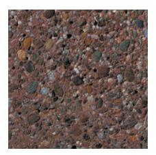
Color: Brown Concrete Color: Gray Texture: Sandblasted Exposure: Medium Description: Fine Aggregate: red/black river sand; Coarse Aggregate: 3/8 to 1/8 in. red/black river gravel; Pigment: red
