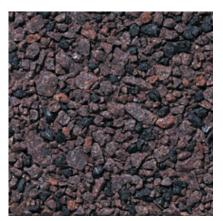
Color: Red Concrete Color: Gray Texture: Retarded Exposure: Medium Description: Fine Aggregate: crushed mauve granite; Coarse Aggregate: 80% - 9/16 to 3/16 in. mauve granite, 20% - 9/16 to 3/16 in. black granite; Pigment: red
