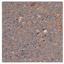
Color: Buff/Tan Concrete Color: Gray Texture: Sandblasted Exposure: Medium Description: Fine Aggregate: brown concrete sand; Coarse Aggregate: 1/2 to 1/4 in. brown river gravel; Pigment: brown
