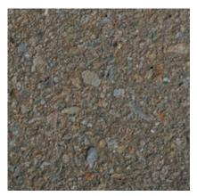
276 Color: Brown Concrete Color: Gray Texture: Sandblasted Exposure: Light Description: Fine Aggregate: crushed tan limestone; Coarse Aggregate: 5/8 to 1/4 in. tan limestone; Pigment: yellow
