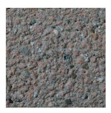
Color: Grey Concrete Color: Gray Texture: Sandblasted Exposure: Light Description: Fine Aggregate: crushed gray granite; Coarse Aggregate: 3/8 to 1/8 in. red granite
