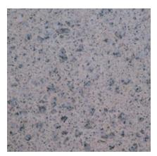
Color: Grey Concrete Color: White Finish: Polished Description: Fine Aggregate: crushed White granite; Coarse Aggregate: 5/8 to 3/32 in. White granite
