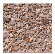
253 Color: Buff/Tan Concrete Color: White Texture: Retarded Exposure: Medium Description: Fine Aggregate: brown masonry sand; Coarse Aggregate: 1/2 to 1/8 in. buff limestone
