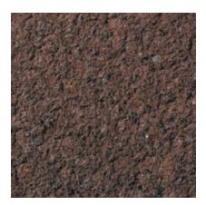
Color: Red Concrete Color: Gray Texture: Sandblasted Exposure: Medium Description: Fine Aggregate: crushed red granite; Coarse Aggregate: 1/2 to 1/4 in. red granite; Pigment: red
