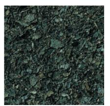
**445** Color: Green Concrete Color: Gray Texture: Retarded Exposure: Light Description: Fine Aggregate: crushed green marble; Coarse Aggregate: 1/2 to 1/8 in. green marble
