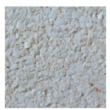
Color: White Concrete Color: White Texture: Retarded Exposure: Light Description: Fine Aggregate: crushed White quartz; Coarse Aggregate: 3/8 to 1/8 in. White quartz
