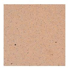
Color: Buff/Tan Concrete Color: 75% - White; 25% - Gray Texture: Sandblasted Exposure: Light Description: Fine Aggregate: crushed White limestone; Coarse Aggregate: 1/2 to 1/4 in. light gray limestone; Pigment: yellow and buff
