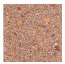
Color: Brown Concrete Color: White Texture: Acid Etched Exposure: Deep Description: Fine Aggregate: buff concrete sand; Coarse Aggregate: 50% - 3/4 to 3/8 in. buff limestone 50% - 3/4 to 3/8 in. brownish red limestone; Pigment: buff
