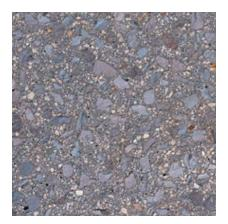
Color: Grey Concrete Color: Gray Texture: Sandblasted Exposure: Medium Description: Fine Aggregate: buff masonry sand; Coarse Aggregate: 1/2 to 1/4 in. reddish brown, limestone; Pigment: dark brown
