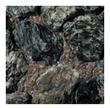
Color: Black - Grey Concrete Color: Gray Finish: Sand Embedment Description: Fine Aggregate: reddish brown concrete sand; Coarse Aggregate: 4 to 2 in. black/gray varigated granite
