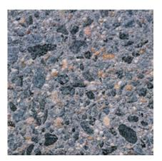
**529** Color: Grey Concrete Color: White Texture: Sandblasted Exposure: Medium Description: Fine Aggregate: White concrete sand; Coarse Aggregate: 1/2 to 1/4 in. gray granite; Pigment: black
