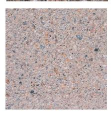
**195** Color: Buff/Tan Concrete Color: Antique White Texture: Sandblasted Exposure: Light Description: Fine Aggregate: crushed salt and pepper granite; Coarse Aggregate: 3/8 to 1/8 in. salt and pepper granite
