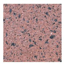
**418** Color: Pink Concrete Color: White Texture: Sandblasted Exposure: Medium Description: Fine Aggregate: crushed orange granite; Coarse Aggregate: 80% - 9/16 to 3/16 in. black granite, 20% - 9/16 to 3/16 in. black granite; Pigment: red
