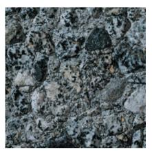
**537** Color: Grey Concrete Color: White Texture: Retarded Exposure: Deep Description: Fine Aggregate: crushed gray granite; Coarse Aggregate: 3/4 to 1/2 in. gray granite; Pigment: black
