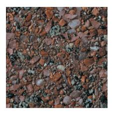
Color: Red Concrete Color: White Texture: Retarded Exposure: Deep Description: Fine Aggregate: crushed gray granite; Coarse Aggregate: 75% - 5/8 to 9/32 in. pink feldspar, 25% - 5/8 to 9/32 in. gray granite; Pigment: red
