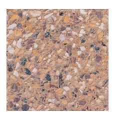
Color: Brown Concrete Color: White Texture: Sandblasted Exposure: Medium Description: Fine Aggregate: buff masonry sand; Coarse Aggregate: 80% - 3/8 to 1/8 in. buff limestone, 20% - 3/8 to 1/8 in. pink quartzite, Pigment: buff
