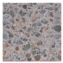
**166** Color: Buff/Tan Concrete Color: 85% - White; 15% - Gray Texture: Sandblasted Exposure: Medium Description: Fine Aggregate: crushed brown granite; Coarse Aggregate: 5/8 to 3/8 in. multicolored, river gravel; Pigment: reddish brown
