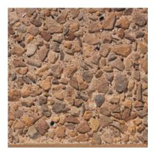
**312** Color: Brown Concrete Color: White Texture: Retarded Exposure: Deep Description: Fine Aggregate: buff masonry sand; Coarse Aggregate: 1/2 to 1/4 in. buff limestone; Pigment: buff
