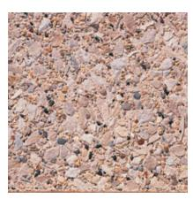
255 Color: Buff/Tan Concrete Color: White Texture: Retarded Exposure: Medium Description: Fine Aggregate: buff concrete sand; Coarse Aggregate: 3/8 to 1/8 in. buff limestone
