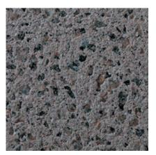
**370** Color: Grey Concrete Color: White Texture: Sandblasted Exposure: Medium Description: Fine Aggregate: crushed gray granite; Coarse Aggregate: 1/2 to 1/4 in. pink granite; Pigment: red
