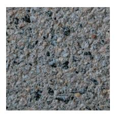
Color: Grey Concrete Color: 50% - White; 50% - Gray Texture: Sandblasted Exposure: Deep Description: Fine Aggregate: crushed gray granite; Coarse Aggregate: 50% - 5/8 to 9/32 in. gray granite, 50% - 1/2 to 1/8 in. pink/black granite
