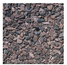
**517** Color: Brown Concrete Color: 50% - Antique White; 50% - Gray Texture: Retarded Exposure: Medium Description: Fine Aggregate: crushed buff limestone; Coarse Aggregate: 1/2 to 1/4 in. gray limestone
