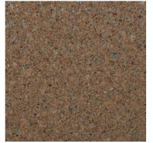
Color: Brown Concrete Color: White Texture: Acid Etched Exposure: Medium Description: Fine Aggregate: reddish brown concrete sand; Coarse Aggregate: 3/8 to 1/8 in. gray granite; Pigment: buff
