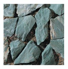
Color: Green Concrete Color: Gray Finish: Sand Embedment Description: Fine Aggregate: reddish brown concrete sand; Coarse Aggregate: 4 to 2 in. green quartzite
