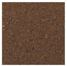
Color: Brown Concrete Color: Gray Texture: Acid Etched Exposure: Light Description: Fine Aggregate: reddish brown concrete sand; Coarse Aggregate: 3/8 to 1/8 in. reddish brown, river gravel; Pigment: buff
