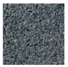
**505** Color: Grey Concrete Color: White Texture: Retarded Exposure: Medium Description: Fine Aggregate: crushed gray granite; Coarse Aggregate: 9/16 to 3/16 in. gray granite; Pigment: black
