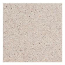
**113** Color: Buff/Tan Concrete Color: White Texture: Sandblasted Exposure: Light Description: Fine Aggregate: buff concrete sand; Coarse Aggregate: 1/2 to 1/4 in. brown limestone; Pigment: buff
