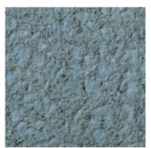
**125** Color: Grey Concrete Color: White Texture: Sandblasted Exposure: Light Description: Fine Aggregate: crushed gray granite; Coarse Aggregate: 5/8 to 9/32 in. White marble
