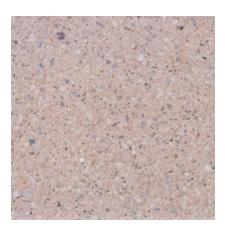
Color: Buff/Tan Concrete Color: White Texture: Acid Etched Exposure: Light Description: Fine Aggregate: crushed White limestone; Coarse Aggregate: 3/8 to 1/8 in. White limestone; Pigment: yellow, brown and black
