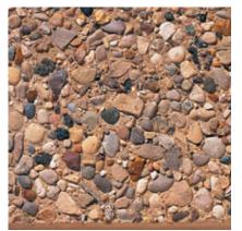
Color: Brown Concrete Color: White Texture: Retarded Exposure: Medium Description: Fine Aggregate: buff concrete sand; Coarse Aggregate: 1/2 to 1/4 in. multicolored river gravel; Pigment: brown
