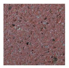
**410** Color: Red Concrete Color: White Texture: Sandblasted Exposure: Light Description: Fine Aggregate: crushed White marble; Coarse Aggregate: 65% - 5/8 to 9/32 in. pink feldspar, 35% - 5/8 to 9/32 in. red granite; Pigment: red
