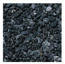
**545A** Color: Black Concrete Color: Gray Texture: Retarded Exposure: Medium Description: Fine Aggregate: crushed black granite; Coarse Aggregate: 1/2 to 1/4 in. black granite; Pigment: black
