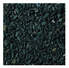
**449** Color: Green Concrete Color: White Texture: Retarded Exposure: Light Description: Fine Aggregate: crushed green marble; Coarse Aggregate: 1/2 to 1/4 in. green marble; Pigment: blue
