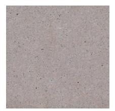
Color: Pink Concrete Color: 50% - White, 50% - Gray Texture: Sandblasted Exposure: Light Description: Fine Aggregate: crushed brown granite ; Coarse Aggregate: 1/2 to 1/4 in. pink granite; Pigment: black
