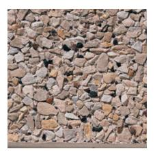
Color: Buff/Tan Concrete Color: White Texture: Retarded Exposure: Deep Description: Fine Aggregate: crushed buff limestone, Coarse Aggregate: 1/2 to 1/4 in. White limestone
