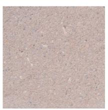
**133** Color: Buff/Tan Concrete Color: antique White Texture: Retarded Exposure: Light Description: Fine Aggregate: crushed buff limestone, Coarse: 1/2 to 1/4 in. buff limestone
