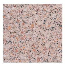
Color: Pink Concrete Color: White Texture: Sandblasted Exposure: Medium Description: Fine Aggregate: buff concrete sand; Coarse Aggregate: 50% - 1/2 to 1/4 in. brownish red limestone 50% - 3/8 to 1/8 in. White limestone
