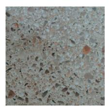
**559** Color: Pink Concrete Color: White Finish: Polished Description: Fine Aggregate: crushed flamingo quartz; Coarse Aggregate: 5/8 to 1/8 in. flamingo quartz
