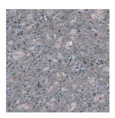
Color: Grey Concrete Color: 50% - White; 50% - Gray Texture: Sandblasted Exposure: Medium Description: Fine Aggregate: crushed black granite; Coarse Aggregate: 1/2 to 1/4 in. salt and pepper granite
