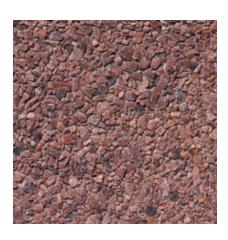
Color: Pink Concrete Color: Antique White Texture: Retarded Exposure: Light Description: Fine Aggregate: crushed pink quartzite; Coarse Aggregate: 3/8 to 1/4 in. pink quartzite; Pigment: red
