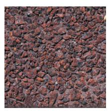
**459** Color: Red Concrete Color: Gray Texture: Retarded Exposure: Medium Description: Fine Aggregate: 80% - buff masonry sand, 20% - crushed red granite; Coarse Aggregate: 9/16 to 3/16 in. red granite; Pigment: red
