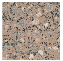
Color: Yellow Concrete Color: Antique White Texture: Sandblasted Exposure: Medium Description: Fine Aggregate: 87% - crushed buff limestone, 13% - black granite grit; Coarse Aggregate: 67% - 1/2 to 1/4 in. pink granite, 22% - 1/2 to 1/4 in. buff limestone, 11% - 1/2 to 1/4 in. black granite; Pigment: red
