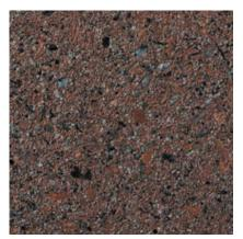
**402** Color: Red Concrete Color: White Texture: Acid Etched Exposure: Deep Description: Fine Aggregate: crushed gray granite; Coarse Aggregate: 75% - 5/8 to 9/32 in. pink feldspar, 25% - 5/8 to 9/32 in. gray granite; Pigment: red
