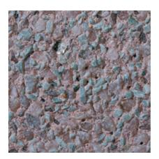
Color: Pink Concrete Color: White Texture: Sandblasted Exposure: Medium Description: Fine Aggregate: crushed flamingo quartz; Coarse Aggregate: 80% - 5/8 to 9/32 in. flamingo quartz, 20% - 9/32 to 1/8 in. green quartzite; Pigment: red
