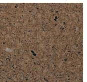
309 Color: Brown Concrete Color: White Texture: Acid Etched Exposure: Medium Description: Fine Aggregate: reddish brown concrete sand; Coarse Aggregate: 3/8 to 1/8 in. reddish brown river gravel; Pigment: 50% brown; 50% yellow
