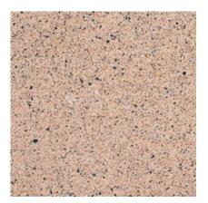
**189** Color: Buff/Tan Concrete Color: White Texture: Sandblasted Exposure: Light Description: Fine Aggregate: buff concrete sand, Coarse Aggregate: 3/4 to 3/8 in. buff marble
