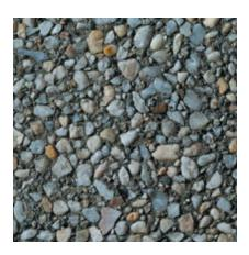
Color: Grey Concrete Color: Gray Texture: Retarded Exposure: Medium Description: Fine Aggregate: crushed gray granite; Coarse Aggregate: 1/2 to 1/4 in. White quartz
