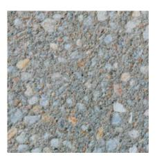
**177** Color: Grey Concrete Color: Gray Texture: Sandblasted Exposure: Deep Description: Fine Aggregate: brown river sand; Coarse Aggregate: 3/4 to 1/2 in. White river gravel; Pigment: brown
