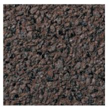
**398** Color: Pink Concrete Color: White Texture: Sandblasted Exposure: Light Description: Fine Aggregate: crushed orange granite; Coarse Aggregate: 3/8 to 1/8 in. orange granite; Pigment: buff
