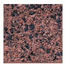
Color: Red Concrete Color: White Texture: Retarded Exposure: Medium Description: Fine Aggregate: crushed orange granite; Coarse Aggregate: 80% - 9/16 to 3/16 in. black granite, 20% - 9/16 to 3/16 in. black granite; Pigment: red
