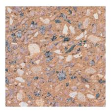
**331** Color: Buff/Tan Concrete Color: White Texture: Sandblasted Exposure: Medium Description: Fine Aggregate: buff masonry sand; Coarse Aggregate: 40% - 1/2 to 1/4 in. buff limestone, 20% - 3/8 to 1/8 in. White limestone, 20% - 3/8 to 1/8 in. pink quartzite, 20% - 3/8 to 1/8 in. black granite; Pigment: buff
