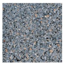
**563** Color: Grey Concrete Color: White Finish: Polished Description: Fine Aggregate: crushed black granite; Coarse Aggregate: 3/8 to 1/8 in. black granite; Pigment: gray
