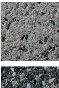
Color: Black - Grey Concrete Color: Gray Texture: Sandblasted Exposure: Medium Description: Fine Aggregate: crushed gray granite; Coarse Aggregate: 75% - 5/8 to 9/32 in. gray granite, 25% - 5/8 to 9/32 in. black granite
