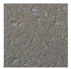
Color: Grey Concrete Color: 70% - Gray; 30% - White Texture: Sandblasted Exposure: Medium Description: Fine Aggregate: crushed reddish brown limestone; Coarse Aggregate: 5/8 to 9/32 in. reddish brown limestone
