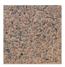
Color: Brown Concrete Color: White Texture: Retarded Exposure: Medium Description: Fine Aggregate: buff masonry sand; Coarse Aggregate: 3/8 to 1/8 in. buff limestone; Pigment: buff
