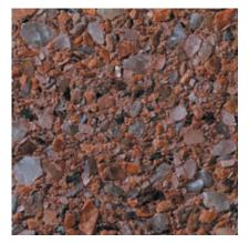
Color: Pink Concrete Color: White Texture: Retarded Exposure: Medium Description: Fine Aggregate: crushed pink feldspar ; Coarse Aggregate: 7/8 to 9/32 in. pink feldspar; Pigment: red
