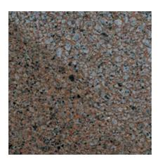
Color: Grey Concrete Color: White Finish: Polished Texture: Acid Etched Description: Fine Aggregate: crushed pink feldspar; Coarse Aggregate: 7/16 to 1/4 in. pink granite; Pigment: 50% - buff; 50% - brown
