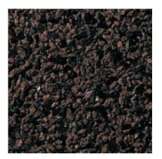
**425** Color: Red - Black Concrete Color: Gray Texture: Retarded Exposure: Light Description: Fine Aggregate: crushed red granite; Coarse Aggregate: 80% - 9/32 to 1/8 in. red granite, 20% - 9/32 to 1/8 in. black granite
