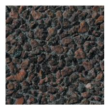
**433** Color: Red Concrete Color: White Texture: Retarded Exposure: Medium Description: Fine Aggregate: crushed gray granite; Coarse Aggregate: 75% - 5/8 to 9/32 in. red granite, 25% - 5/8 to 9/32 in. light red granite; Pigment: black
