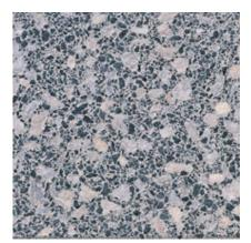
**162** Color: Black Concrete Color: White Texture: Sandblasted Exposure: Medium Description: Fine Aggregate: 95% - crushed black granite sand, 5% - White silica sand; Coarse Aggregate: 5/8 to 1/4 in. White limestone
