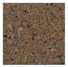
Color: Brown Concrete Color: White Texture: Acid Etched Exposure: Deep Description: Fine Aggregate: reddish brown concrete sand, Coarse Aggregate: 1/2 in. reddish brown river gravel, Pigment: yellow
