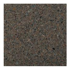
Color: Brown Concrete Color: Gray Texture: Acid Etched Exposure: Medium Description: Fine Aggregate: reddish brown masonry sand; Coarse Aggregate: 1/2 to 1/4 in. reddish brown river gravel
