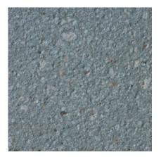
229 Color: Grey Concrete Color: Gray Texture: Sandblasted Exposure: Medium Description: Fine Aggregate: crushed gray limestone; Coarse Aggregate: 1/2 in. gray limestone
