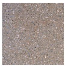
225 Color: Brown Concrete Color: White Finish: Honed Exposure: Medium Description: Fine Aggregate: crushed White limestone; Coarse Aggregate: 3/8 to 1/8 in. White limestone; Pigment: ocher and green
