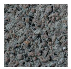
Color: Grey Concrete Color: 50% - White; 50% - Gray Texture: Sandblasted Exposure: Medium Description: Fine Aggregate: crushed gray granite; Coarse Aggregate: 75% - 1/2 to 1/4 in. pink granite, 25% - 5/8 to 9/32 in. gray granite
