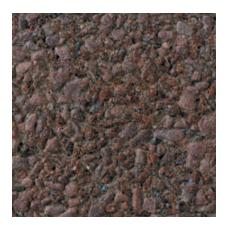
Color: Red Concrete Color: Gray Texture: Sandblasted Exposure: Medium Description: Fine Aggregate: reddish brown concrete sand; Coarse Aggregate: 50% - 3/8 to 1/8 in. pink quartz, 50% - 3/8 to 1/8 in. red granite
