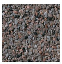
**455** Color: Pink Concrete Color: Gray Texture: Retarded Exposure: Light Description: Fine Aggregate: crushed red quartzite; Coarse Aggregate: 60% - 3/8 to 1/8 in. pink feldspar, 30% - 3/8 to 1/8 in. black granite, 10% - 3/8 to 1/8 in. red quartzite
