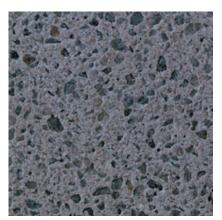
**173** Color: Grey Concrete Color: White Texture: Sandblasted Exposure: Medium Description: Fine Aggregate: crushed gray quartz; Coarse Aggregate: 3/8 to 1/8 in. gray quartz
