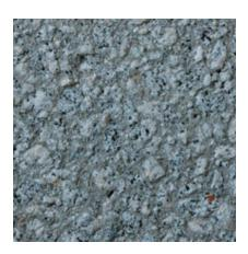
Color: Grey Concrete Color: Gray Texture: Sandblasted Exposure: Medium Description: Fine Aggregate: crushed gray granite; Coarse Aggregate: 3/8 to 1/4 in. gray granite
