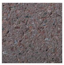
**378** Color: Pink Concrete Color: Gray Texture: Sandblasted Exposure: Medium Description: Fine Aggregate: crushed gray granite; Coarse Aggregate: 60% - 1/2 to 1/4 in. gray granite, 40% - 9/32 to 1/8 in. red quartzite; Pigment: red
