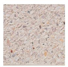
Color: White Concrete Color: White Texture: Retarded Exposure: Medium Description: Fine Aggregate: crushed White quartz; Coarse Aggregate: 9/16 to 3/16 in. White quartz; Pigment: White
