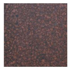
**567** Color: Red Concrete Color: Gray Finish: Polished Description: Fine Aggregate: crushed black granite; Coarse Aggregate: 1/2 to 3/8 in. red granite; Pigment: 50% - brown; 50% - orange/red
