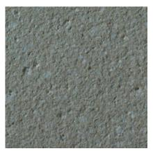
221 Color: Brown Concrete Color: White Texture: Sandblasted Exposure: Medium Description: Fine Aggregate: crushed gray limestone; Coarse Aggregate: 1/2 in. gray limestone; Pigment: dark buff
