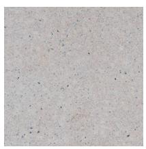
**127** Color: Buff/Tan Concrete Color: White Texture: Acid Etched Exposure: Light Description: Fine Aggregate: 90% - White river sand, 10% - crushed black granite; Coarse Aggregate: 1/2 to 1/4 in. black granite
