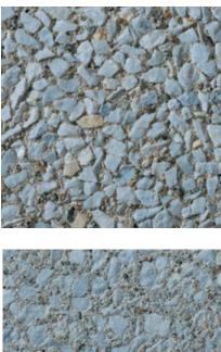
Color: White Concrete Color: White Texture: Retarded Exposure: Medium Description: Fine Aggregate: crushed gray granite, Coarse Aggregate: 1/2 to 3/8 in. White marble
