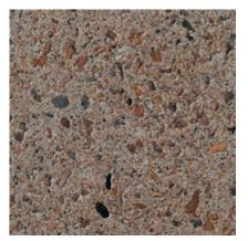
241 Color: Red Concrete Color: White Texture: Acid Etched Exposure: Deep Description: Fine Aggregate: reddish brown concrete sand; Coarse Aggregate: 3/8 to 1/8 in. reddish brown river gravel
