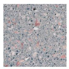
Color: Pink Concrete Color: 50% - White; 50% - Gray Texture: Sandblasted Exposure: Medium Description: Fine Aggregate: crushed gray quartz; Coarse Aggregate: 75% - 1/2 to 1/4 in. pink feldspar, 25% - 1/2 to 1/4 in. White marble
