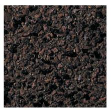
Color: Red Concrete Color: Gray Texture: Retarded Exposure: Medium Description: Fine Aggregate: reddish brown masonry sand; Coarse Aggregate: 80% - 5/8 to 9/32 in. red granite, 20% - 9/32 to 1/8 in. black granite; Pigment: red
