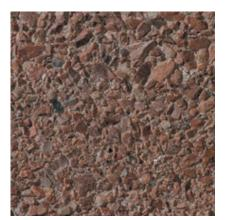
265 Color: Pink Concrete Color: White Texture: Retarded Exposure: Medium Description: Fine Aggregate: crushed pink feldspar, Coarse Aggregate: 1/2 to 1/4 in. pink feldspar
