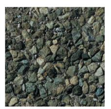
**441** Color: Green Concrete Color: Gray Texture: Retarded Exposure: Deep Description: Fine Aggregate: crushed gray granite; Coarse Aggregate: 1/2 to 1/4 in. green marble
