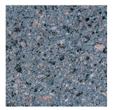
291B Color: Grey Concrete Color: Gray Texture: Sandblasted Exposure: Light Description: Fine Aggregate: crushed red granite; Coarse Aggregate: 1/2 to 1/8 in. red granite; Pigment: black
