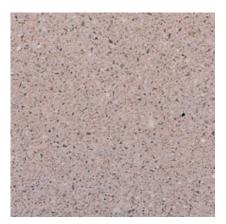
**137** Color: Buff/Tan Concrete Color: White Finish: Honed Description: Fine Aggregate: crushed White limestone; Coarse Aggregate: 3/8 to 1/8 in. White limestone; Pigment: yellow, brown and black
