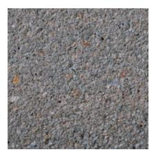
Color: Grey Concrete Color: Gray Texture: Acid Etched Exposure: Light Description: Fine Aggregate: crushed gray granite; Coarse Aggregate: 9/32 to 1/8 in. gray granite
