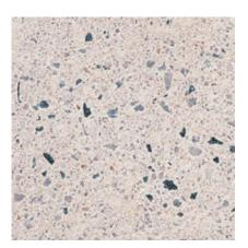
205 Color: White Concrete Color: White Texture: Sandblasted Exposure: Medium Description: Fine Aggregate: crushed gray quartz; Coarse Aggregate: 90% - 1/2 to 1/4 in. gray quartz, 10% - 3/8 to 1/8 in. black granite
