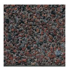
Color: Red Concrete Color: Gray Texture: Retarded Exposure: Medium Description: Fine Aggregate: crushed buff limestone; Coarse Aggregate: 70% - 9/16 to 3/16 in. red granite, 30% - 3/8 to 1/8 in. black granite
