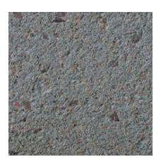
Color: Grey Concrete Color: White Texture: Sandblasted Exposure: Light Description: Fine Aggregate: reddish brown concrete sand; Coarse Aggregate: 60% - 5/8 to 9/32 in. red quartzite, 40% - 5/8 to 9/32 in. gray granite; Pigment: black
