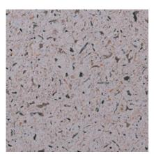
165 Color: Pink Concrete Color: White Texture: Acid Etched Exposure: Medium Description: Fine Aggregate: crushed rose quartz; Coarse Aggregate: 5/8 to 9/32 in. rose quartz
