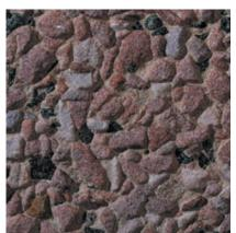
Color: Red Concrete Color: Gray **Texture:** Sandblasted Exposure: Medium **Description:** Fine Aggregate: crushed red quartzite; Coarse Aggregate: 70% - 5/8 to 9/32 in. red quartzite, 30% - 5/8 to 9/32 in. black granite
