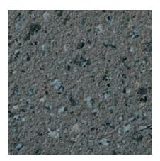
Color: Grey Concrete Color: Gray Texture: Sandblasted Exposure: Light Description: Fine Aggregate: crushed gray granite; Coarse Aggregate: 1/2 to 3/8 in. gray granite
