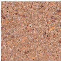
Color: Buff/Tan Concrete Color: White Texture: Acid Etched Exposure: Medium Description: Fine Aggregate: buff concrete sand; Coarse Aggregate: 3/4 to 1/8 in. buff limestone ; Pigment: buff
