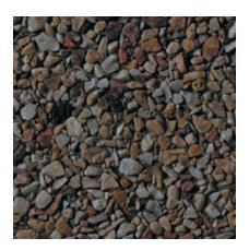
Color: Brown Concrete Color: Gray Texture: Retarded Exposure: Light Description: Fine Aggregate: crushed brown limestone; Coarse Aggregate: 3/8 to 1/8 in. brown limestone; Pigment: brown
