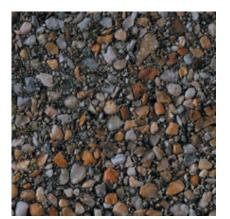
**513** Color: Brown Concrete Color: Gray Texture: Retarded Exposure: Medium Description: Fine Aggregate: crushed gray granite; Coarse Aggregate: 1/2 to 1/4 in. amber quartz
