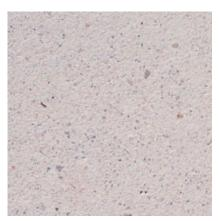
**109** Color: White Concrete Color: White Texture: Sandblasted Exposure: Medium Description: Fine Aggregate: crushed buff limestone; Coarse Aggregate: 1/2 to 1/4 in. buff limestone
