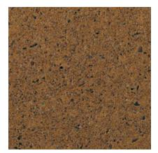
Color: Brown Concrete Color: White Texture: Acid Etched Exposure: Medium Description: Fine Aggregate: reddish brown concrete sand ; Coarse Aggregate: 1/2 to 1/4 in. reddish brown river gravel; Pigment: yellow
