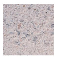
Color: White Concrete Color: White Texture: Sandblasted Exposure: Deep Description: Fine Aggregate: crushed buff limestone; Coarse Aggregate: 1/2 to 1/4 in. buff limestone
