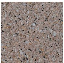
249 Color: Brown Concrete Color: White Texture: Sandblasted Exposure: Medium Description: Fine Aggregate: crushed gray limestone; Coarse Aggregate: 50% - 1/2 in. gray limestone, 40% - coquina shell, 10% - crushed black granite grit; Pigment: 50% dark buff; 50% dark red
