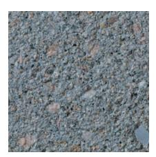
Color: Grey Concrete Color: White Texture: Sandblasted Exposure: Light Description: Fine Aggregate: crushed gray granite; Coarse Aggregate: 60% - 5/8 to 9/32 in. gray granite, 40% - 5/8 to 9/32 in. pink feldspar; Pigment: black
