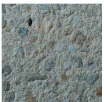
213 Color: White Concrete Color: White Texture: Sandblasted Exposure: Deep Description: Fine Aggregate: White river sand ; Coarse Aggregate: 7/8 to 9/16 in. White river gravel
