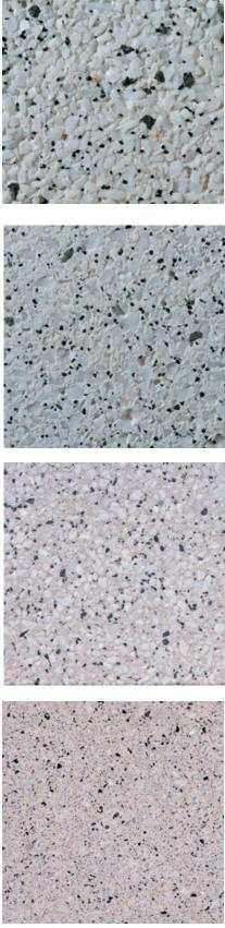
Color: White Concrete Color: White Texture: Retarded **Exposure:** Medium **Description:** Fine Aggregate: crushed White quartz; Coarse Aggregate: 80% - 3/8 to 1/8 White quartz, 10% - 3/8 to 1/8 in. black granite, 10% - black slag
