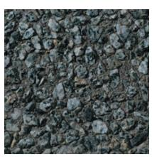
**515** Color: Grey Concrete Color: Gray Texture: Retarded Exposure: Medium Description: Fine Aggregate: crushed gray granite; Coarse Aggregate: 1/2 to 3/8 in. gray granite
