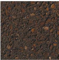
Color: Brown Concrete Color: White Texture: Sandblasted Exposure: Medium Description: Fine Aggregate: reddish brown masonry sand; Coarse Aggregate: 1/2 to 1/4 in. brown river gravel; Pigment: brown
