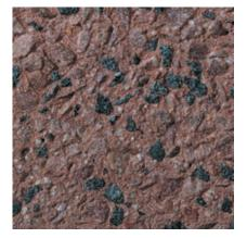
Color: Pink Concrete Color: 50% - White; 50% - Gray Texture: Sandblasted Exposure: Medium Description: Fine Aggregate: White silica concrete sand; Coarse Aggregate: 80% - 1/2 to 1/4 in. pink quartzite, 20% - 1/2 to 1/4 in. black granite; Pigment: 50% red; 50% brown
