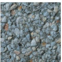
209 Color: Grey Concrete Color: Gray Texture: Sandblasted Exposure: Medium Description: Fine Aggregate: crushed gray granite; Coarse Aggregate: 1/2 to 1/4 in. White quartz
