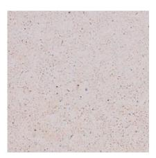
141 Color: White Concrete Color: White Texture: Acid Etched Exposure: Light Description: Fine Aggregate: crushed White marble; Coarse Aggregate: 1/2 to 1/4 in. White/buff marble
