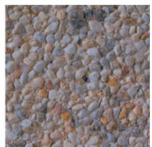
**178** Color: White Concrete Color: White Texture: Retarded Exposure: Medium Description: Fine Aggregate: White river sand; Coarse Aggregate: 1/2 to 3/8 in. White river gravel
