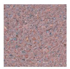
Color: Pink Concrete Color: Gray Texture: Sandblasted Exposure: Medium Description: Fine Aggregate: 80% - buff masonry sand, 20% - crushed red granite; Coarse Aggregate: 9/16 to 3/16 in. red granite; Pigment: red
