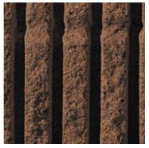
**575** Color: Brown Concrete Color: White Finish: Fine Stone Rib Description: Fine Aggregate: reddish brown concrete sand, Coarse Aggregate: 3/8 to 1/8 in. reddish brown river gravel; Pigment: yellow
