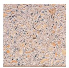
Color: Buff/Tan Concrete Color: White Texture: Sandblasted Exposure: Medium Description: Fine Aggregate: buff concrete sand, Coarse Aggregate: 3/4 to 3/8 in. buff marble
