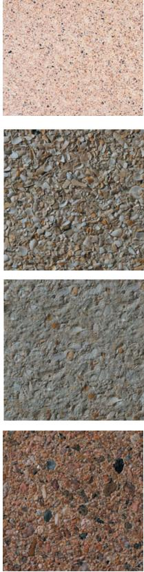
Color: Buff/Tan Concrete Color: White Texture: Acid Etched Exposure: Medium Description: Fine Aggregate: buff concrete sand; Coarse Aggregate: 3/8 to 1/8 in. buff limestone
