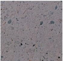
217 Color: White Concrete Color: White Texture: Sandblasted Exposure: Light Description: Fine Aggregate: White masonry sand; Coarse Aggregate: 1/2 to 1/4 in. White river gravel
