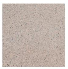
**157** Color: Buff/Tan Concrete Color: White Texture: Acid Etched Exposure: Light Description: Fine Aggregate: off-White river sand, Coarse Aggregate: 1/2 to 1/4 in. black granite, Pigment: dark buff
