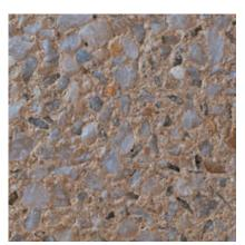
**185** Color: White Concrete Color: White Texture: Sandblasted Exposure: Medium Description: Fine Aggregate: crushed White quartz, Coarse Aggregate: 80% - 5/8 to 9/32 in. White quartz, 20% - 1/2 to 1/4 in. amber quartz; Pigment: yellow
